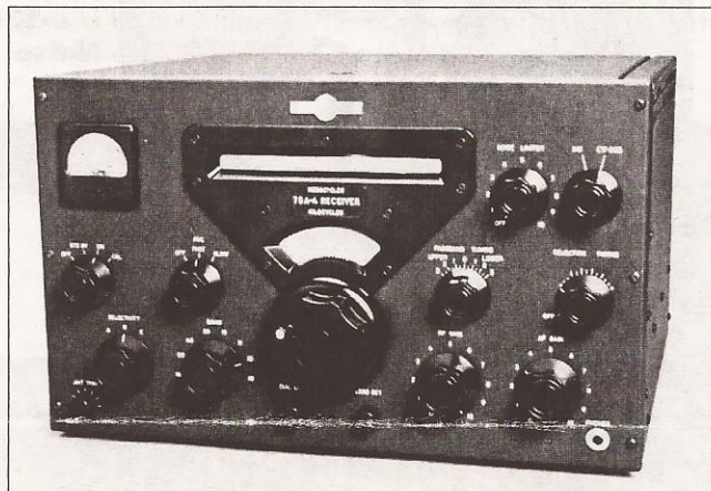
Figure 1 The 75A-4 was the first commercial single sideband amateur receiver. It remains probably one of the most prized possessions of any Collins enthusiast.
