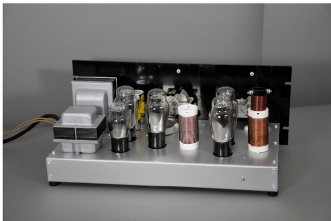
Restoring the chassis and transformers in place was tedious and tricky. The chassis end plates and topside exposed screws were all restored using original finishes which were a combination of nickel and cadmium plating. All of the other components were simply carefully cleaned with no other enhancements. Upon reassembly, every move was carefully calculated to ensure no damage to any surface. The nitty-gritty details of this restoration are a story all in itself.
