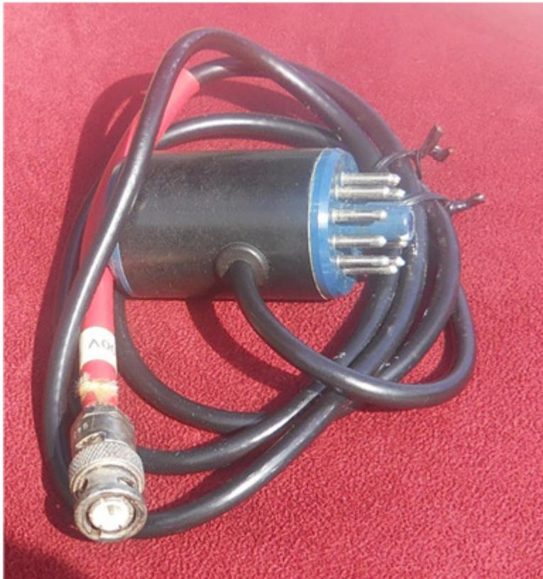
Assembly of the tubular adapter is best done by starting at the female end and bring everything through including the 800 V tap and shield and then by running all of the properly stripped “through wires” out through the unsoldered male pins. Then finish it off by soldering all of the male pins.
